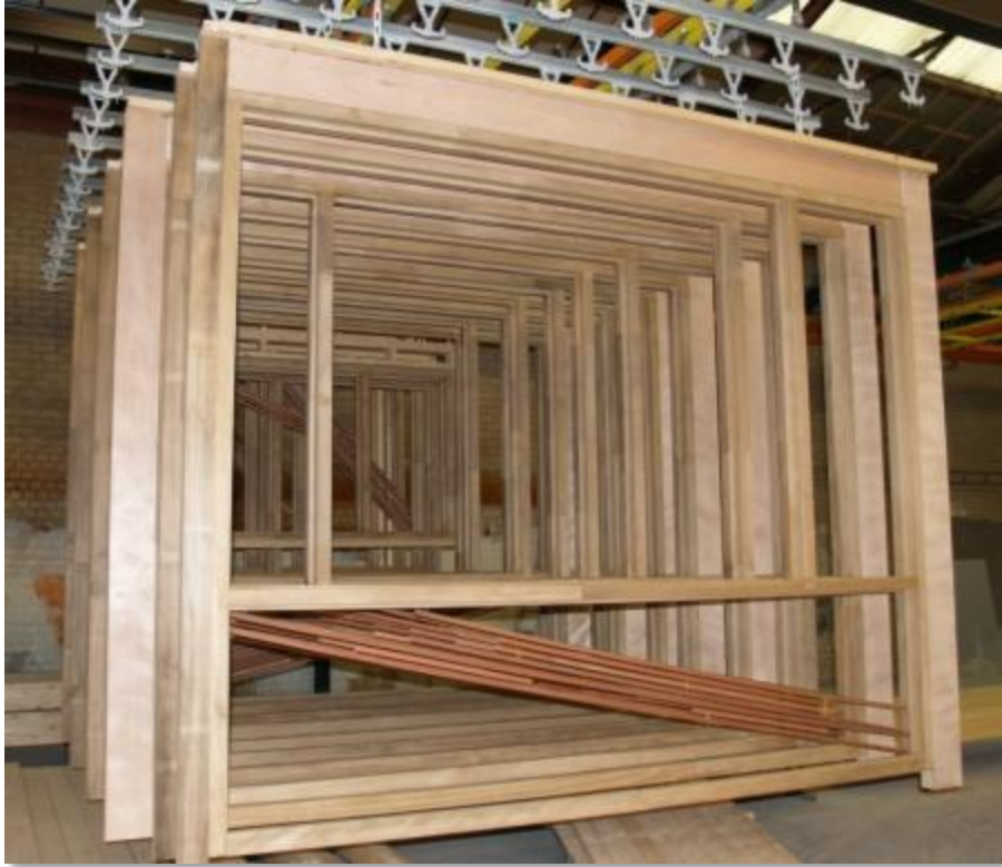
Finger-jointed acetylated wood used to manufacture windows
