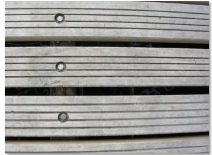
Acetylated wood decking after 1 year exposure (Uncoated)
